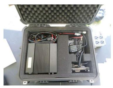
pick a apart foam inside the case works great to form around the radio gear. As you can see in the photos how it is packed away for transport and then how it is set up for deployment. Combine this go box with the Arrow J Pole antenna I had on the my Buddipole mast I showed you guys in the September newsletter and you can have a complete VHF, UHF EMCOMM portable station that can be set up in minute.
