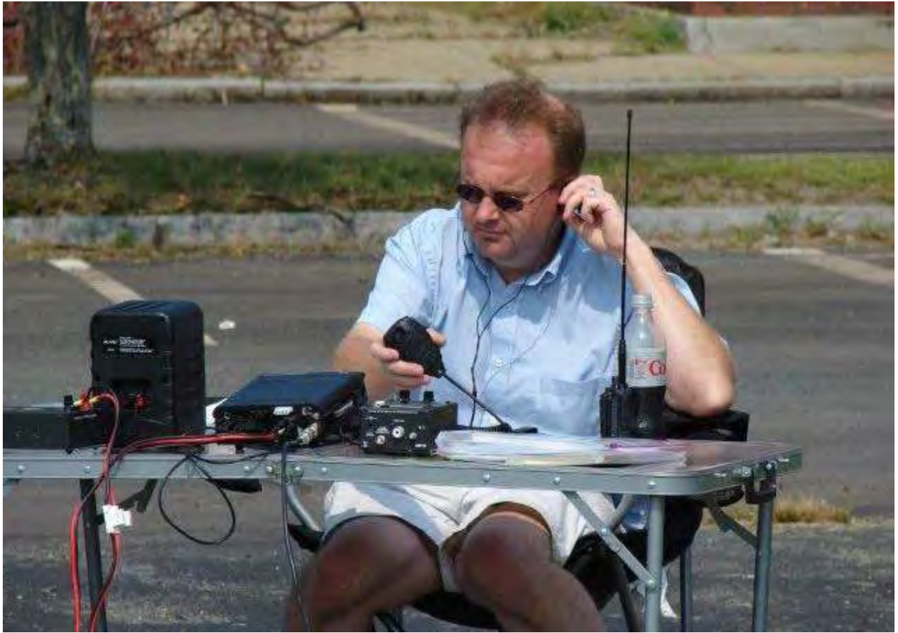
Deana setup his Yaesu FT817 QRP rig and his trusty Buddipole Antenna system
