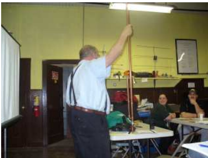
Curtis with a homebrew J-Pole constructed from common copper plumbing pipe.
