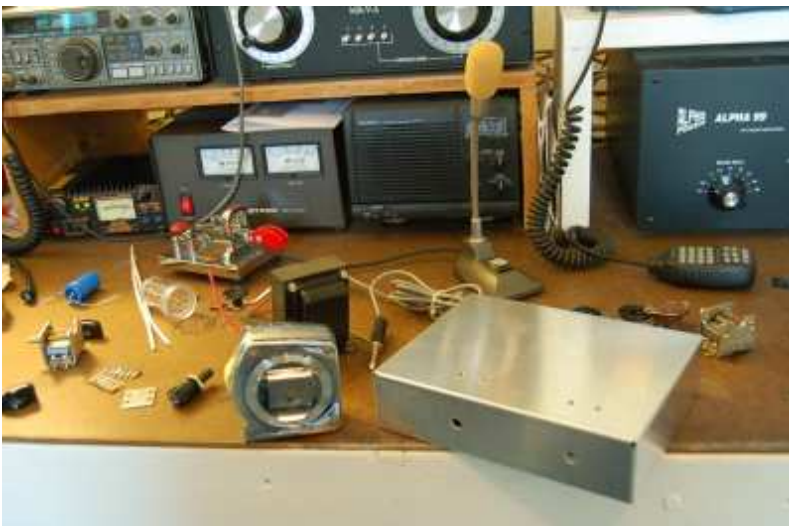
I started by punching and drilling for the variable caps.
