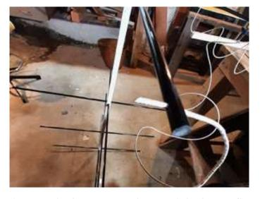
The coax is then wrapped around the boom five or six times and taped in place.
