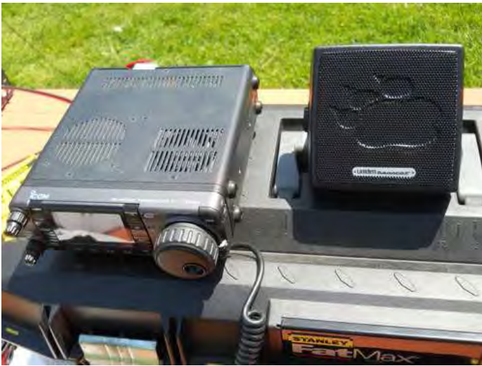
A picture of the Icom 7000 with the Uniden Speaker to compare the size of the speaker to the rig.
