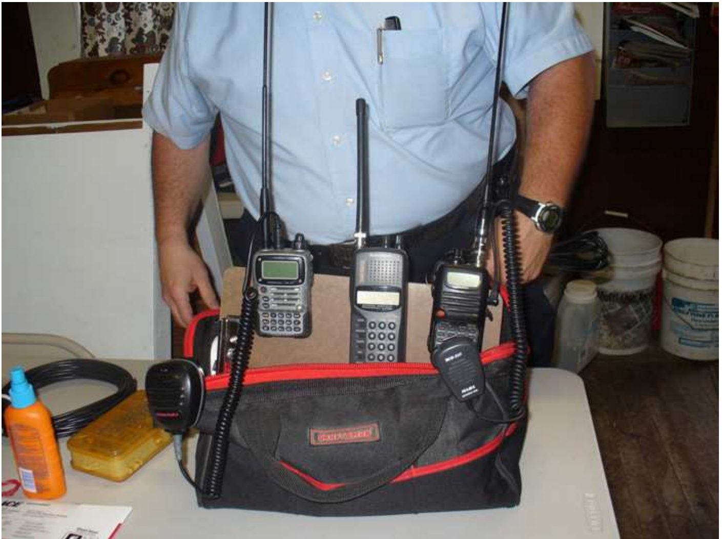
The two pics are the Emcomm group relaying simulated damage assessment message traffic from Bill Canty-W1OKD in Manchester and passing it on to Hurricane Net Control and the bag with the two radios and scanner are Chuck Downey`s- N1OCT portable Emcomm Go-kit. Courtesy Dean-PGH
