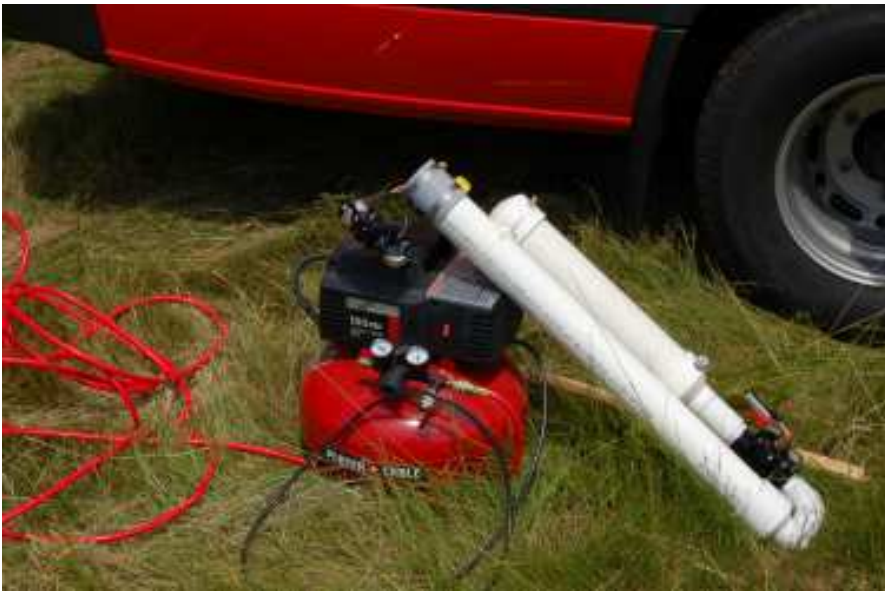
The K1TP tennis ball launcher was effective for installing the dipole antennas.
