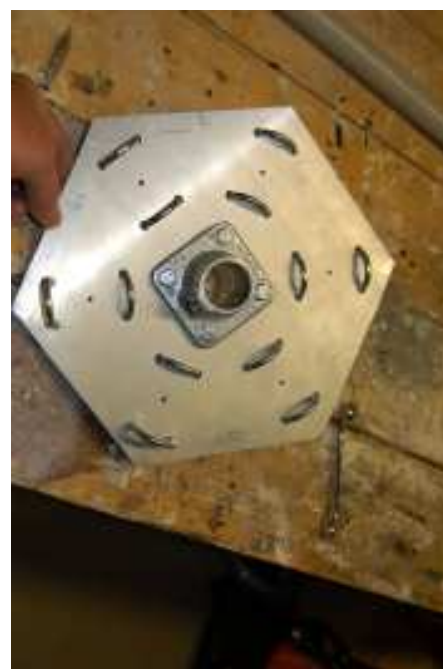
The base all drilled and assembled with clamps and pipe flange
