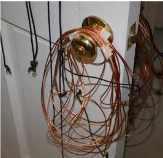
A set of director and reflector wires are made from Davis-RF "Flexweave" copper wire for each band.
