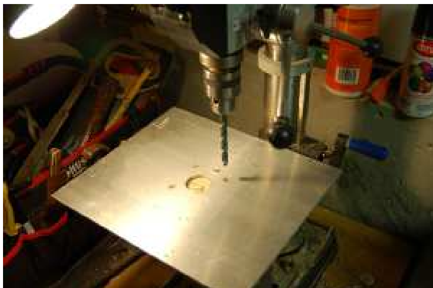
The photo above show the 3/16 thick aluminum plate as I started drilling and cutting to the completed hex shape.
