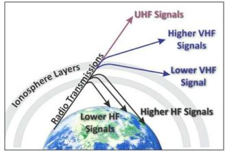
to 30-meters (10 MHz) are often effectively refracted back to earth's surface when directed toward the horizon where incidence angles into the ionosphere are closer to the horizontal, and this propagation geometry provides long skip distances with single skips up to 2500 miles. However, the ionosphere usually does not have sufficient bending strength to return these upper HF band frequencies to earth with the steep take-off angles necessary for the NVIS technique.
