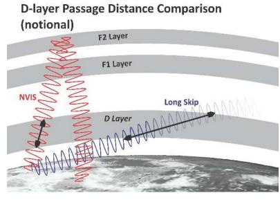
The ionosphere's bending effect is sufficient, even at steep "near vertical" angles of incidence, to bend back to earth the lower HF frequencies, particularly the 40-meter band (7 MHz), 60-meter band (5.3 MHz), and 80-meter band (3.5 MHz) signals. These bands are most suitable for the NVIS technique, even during daylight hours when more distant skip propagation on these bands is ineffective due to D-layer absorption.
