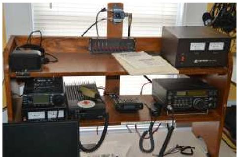
This is a new station setup for vhf and uhf radio operation. With these radios you can work on two or six meters all modes using the 2 and 6 meter beams on the new tower installation.
