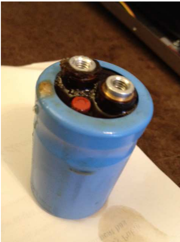
Electrolytic that failed in the 4000 volt power supply section of the HF Amplifier.
