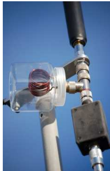
Closeup of the shunt coil I built for easier 80 meter loading
