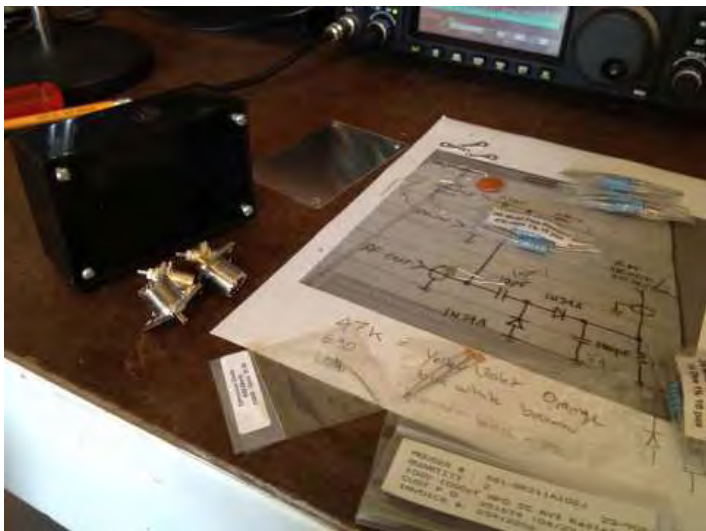
New winter project: An RF sampler so you can watch your rf signal on your oscilloscope. ....K1TP
