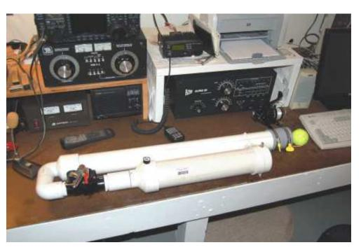
This is the first one that I built which shows the fishing reel attached at the end of the barrel and tennis ball atached to fishing line.
