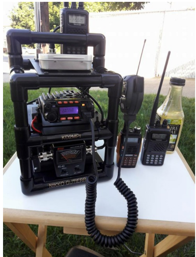
Another idea for a go-kit, this is made from white pvc and spray painted black
