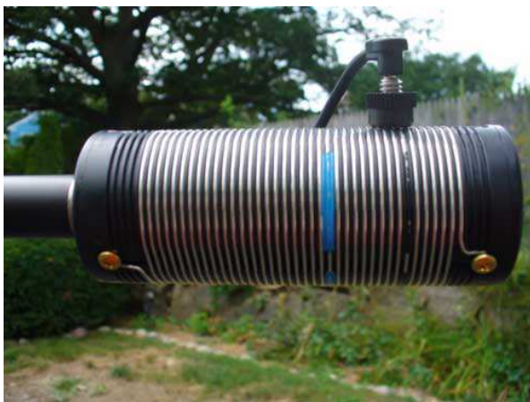
Well constructed coils for quick band switching.
