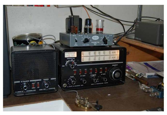
Drake 2B with speaker/qmultiplier and the homebrew Ameco AC-1 clone I built last winter. I made my first contact straight key with a wonderfully chirpy signal to PA on 7040 last week.....Jon-K1TP
