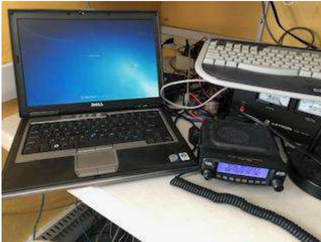
440 WiresX repeater setup
